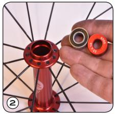
CLEAN BEARING BORE OF ANY DIRT, GREASE OR CONTAMINATION AND FIND CORRECT REPLACEMENT BEARINGS FOR YOUR APPLICA-TION.
