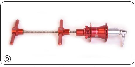
OVER AXLE ADAPTERS USE A QUICK RELEASE SKEWER THAT THREADS INTO THE THREADED PRESS ROD. SPIN THE PRESS HANDLE CLOSEST TO THE HUB TO INSERT BEARING INTO BEARING BORE. QUICK RELEASE SKEWER IS PART OF OUR SMALL SEALED BEARING PRESS (<u>PRESS-2</u>).
