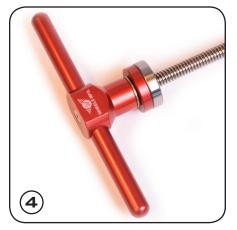
PLACE BEARING ONTO BEARING ADAPTER, ENSURING IT IS SEATED CORRECTLY. INSERT HANDLE WITH BEARING AND ADAPTER INTO HUB. PLACE OPEN BORE ADAPTER ONTO THEADED HANDLE FROM OPPOSITE SIDE, SECURING WITH OTHER HANDLE.
