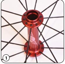
REMOVE OLD/ WORN BEARINGS FROM HUB/ BOTTOM BRACKET WITH WHEELS MFG SEALED BEARING EXTRACTOR SET (<u>PRESS-5</u>) OR APPROPRIATE INDIVIDUAL SEALED BEARING EXTRACTOR.
