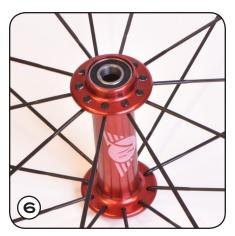
REMOVE HANDLE AND ADAPTER FROM HUB. THE FRST BEARING IS INSTALLED. REPEAT THIS PROCESS FOR THE SECOND BEARING.
